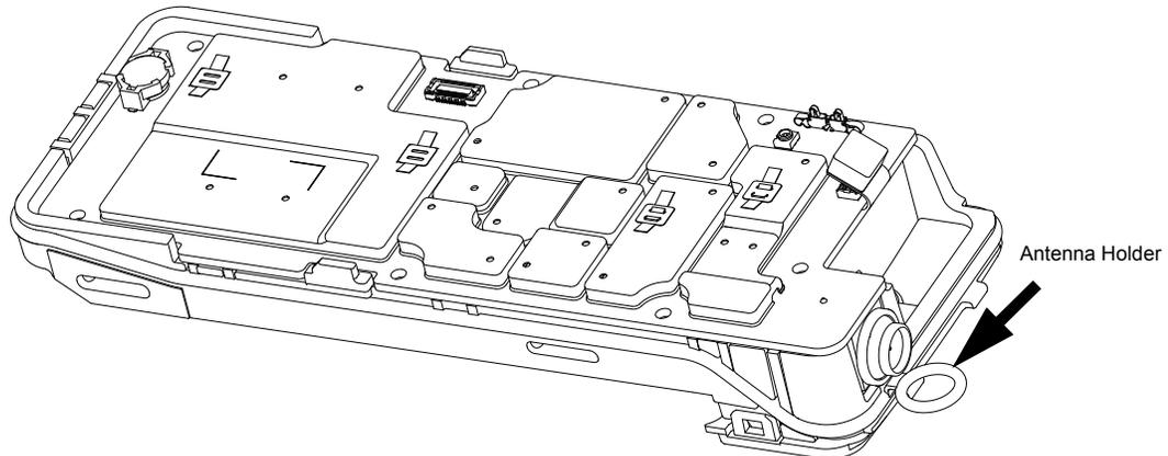
Figure 8-10. Remove the Main O-Ring at the antenna holder
