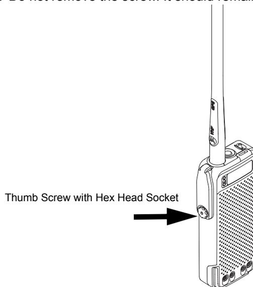
*Figure 8-2. Removing the Thumb Screw*
