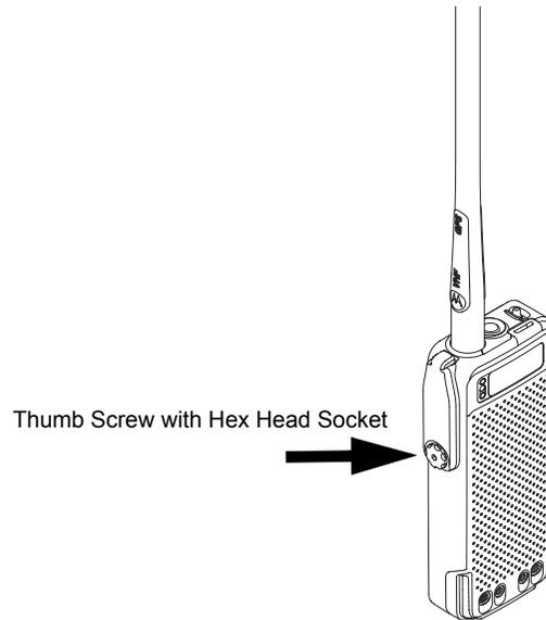
Figure 8-24. Securing the Cover
