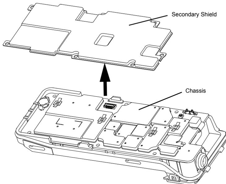
*Figure 8-9. Remove the Secondary Shield Assembly*
