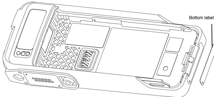
Figure 8-28. Assemble the Bottom Label
