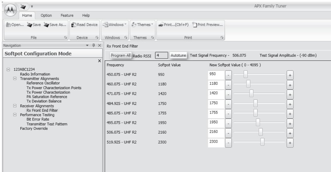
Figure 6-26. Front End Filter Alignment Screen (UHF2)
