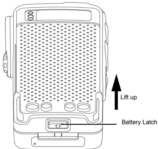
*Figure 8-4. Lifting up the latch*
