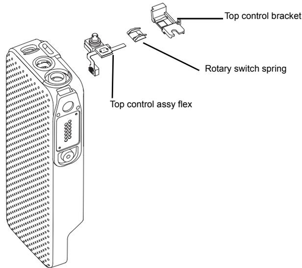
Figure 8-15. Serviceable Components – Main Housing
