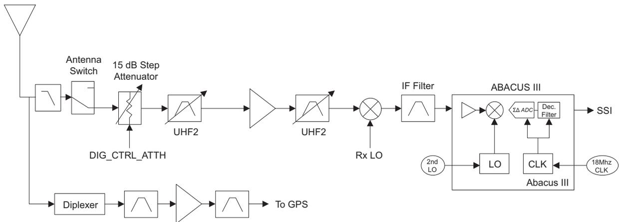
Figure 3-3. Receiver Block Diagram (UHF2)
