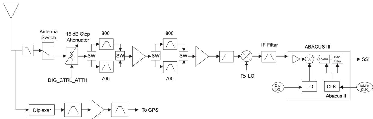
Figure 3-5. Receiver Block Diagram (700/800 MHz)
