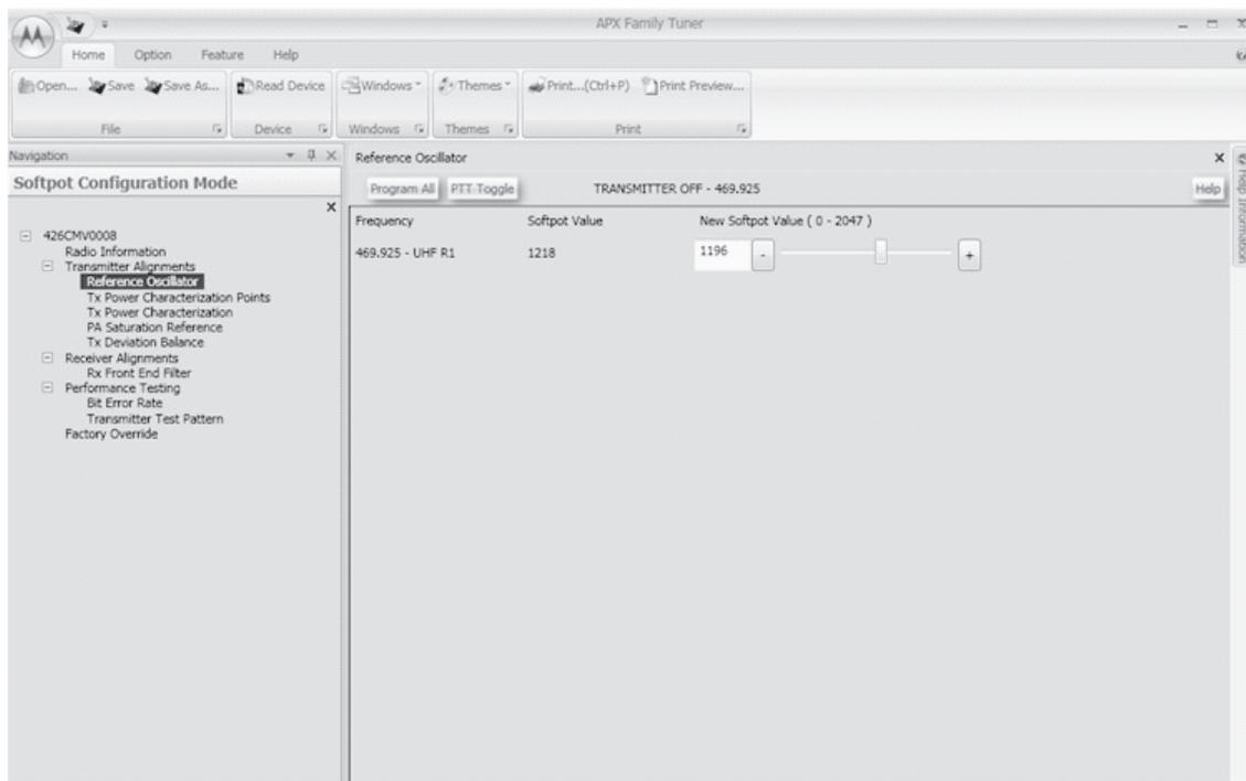
Figure 6-5. Reference Oscillator Alignment Screen (UHF1)
