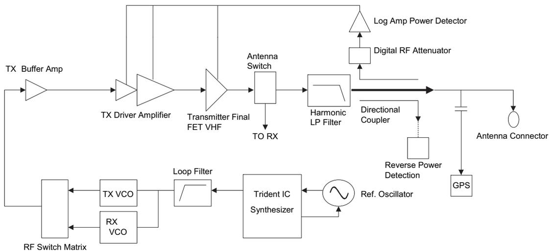
Figure 3-8. Transmitter (VHF) Block Diagram
