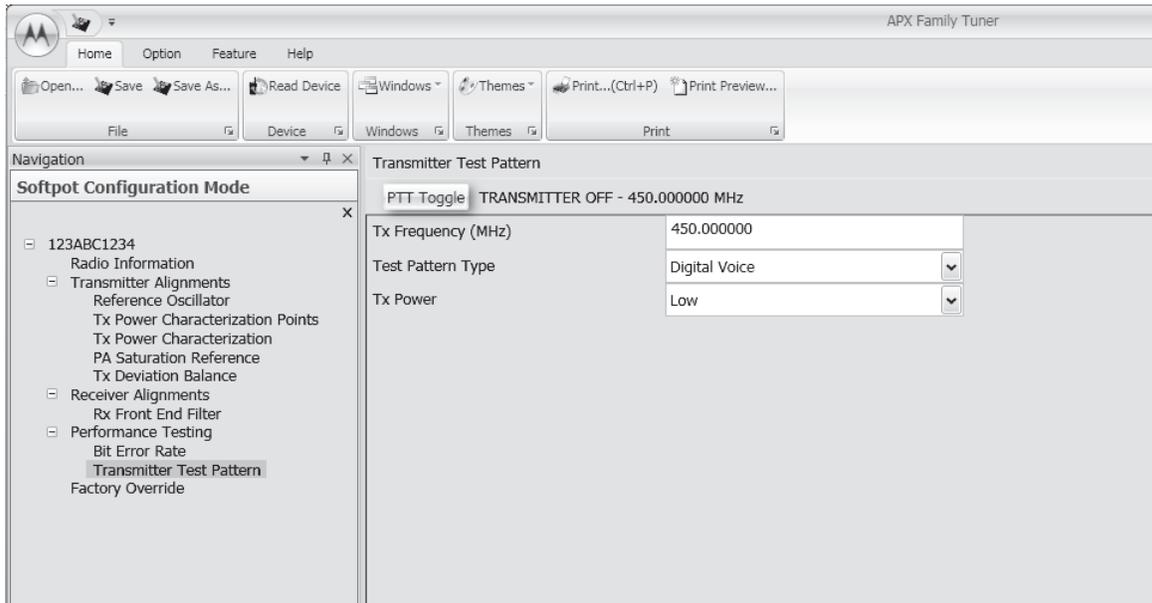
Figure 6-32. Transmitter Test Pattern Screen (UHF2)
