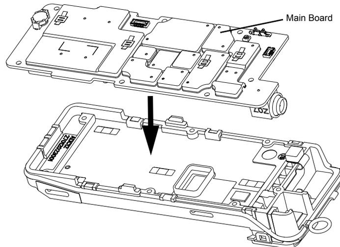
Figure 8-18. Assemble the RF Board
