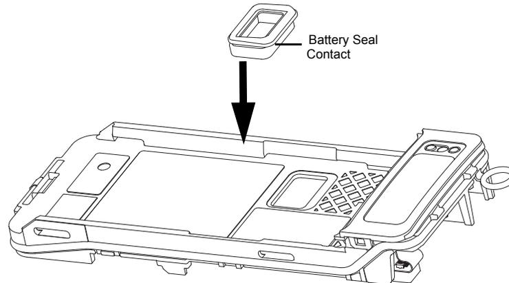
*Figure 8-16. Assemble the Battery Seal*
