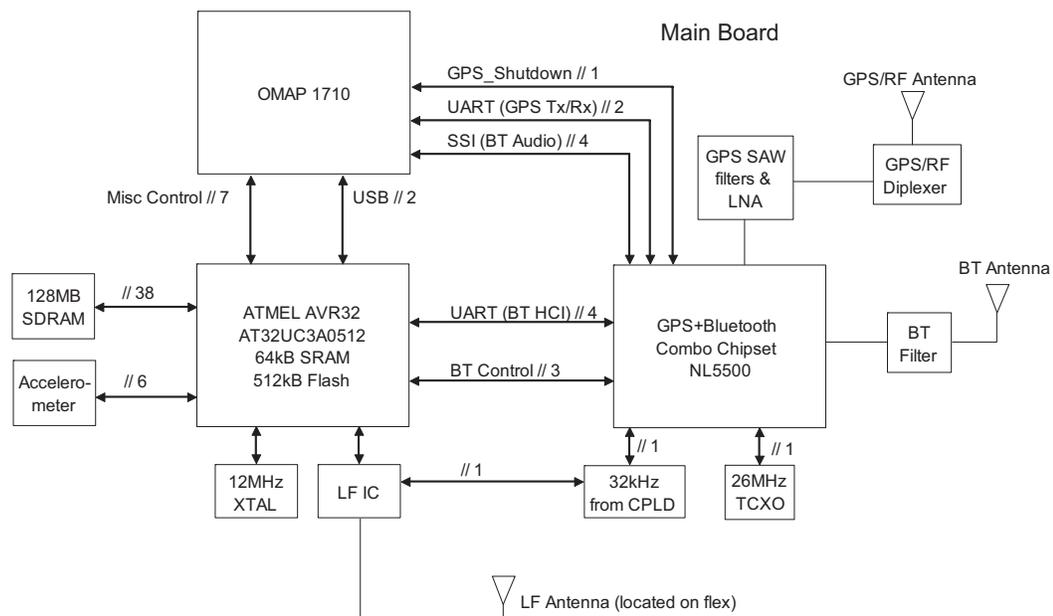
Figure 3-11. GPS/Bluetooth/Accelerometer Block Diagram
