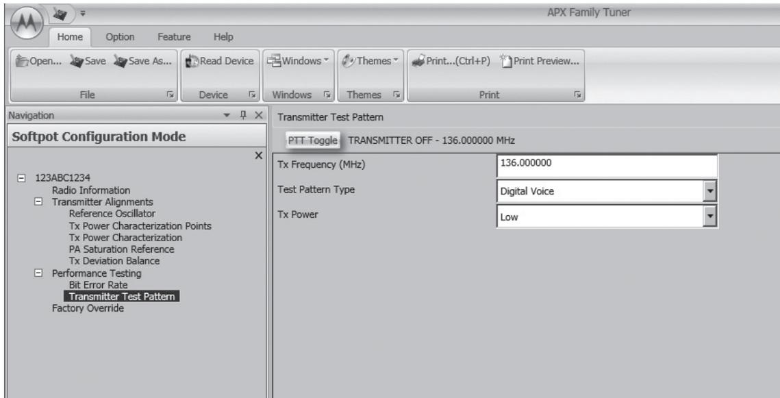
Figure 6-33. Transmitter Test Pattern Screen (VHF)
