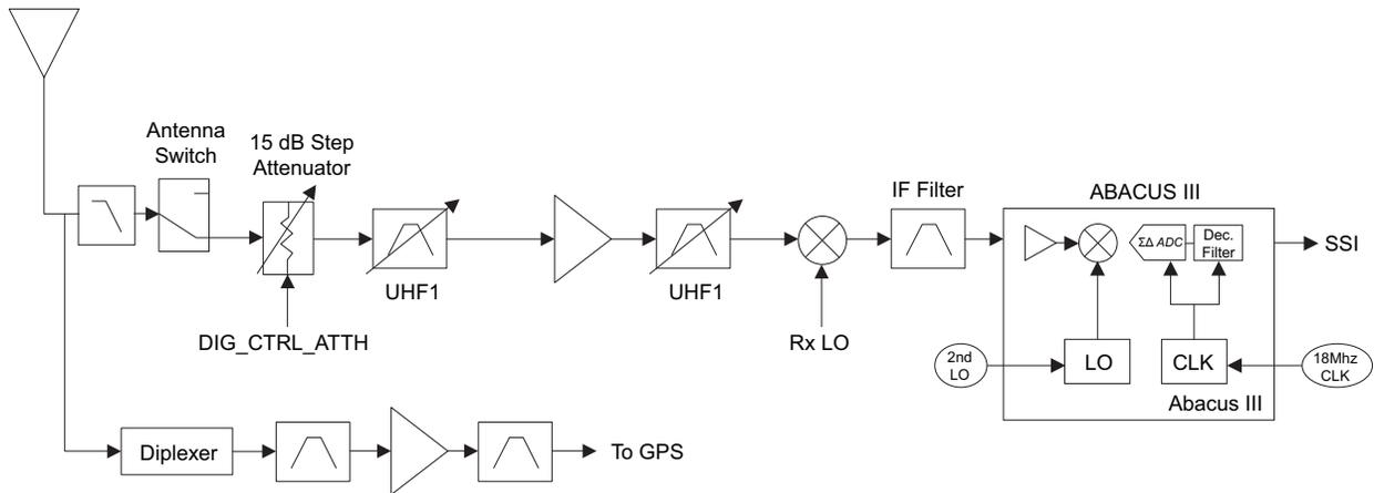
Figure 3-2. Receiver Block Diagram (UHF1)
