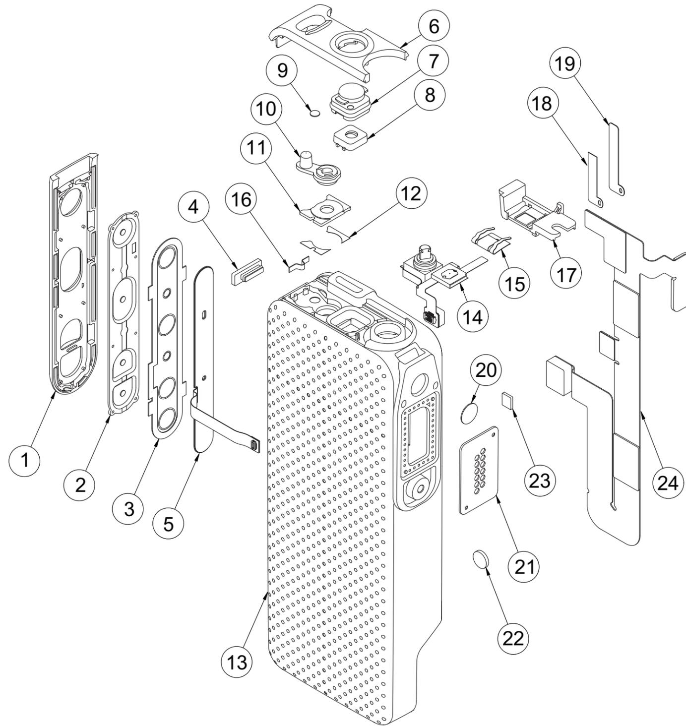
Figure 10-1. APX 3000 Front Kit Exploded View
