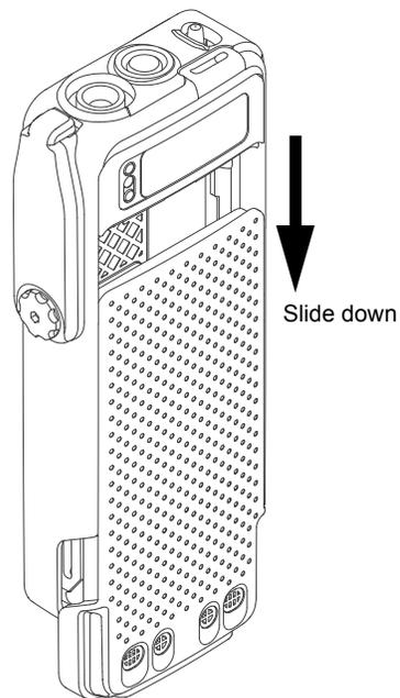
*Figure 8-5. Removing the Battery*
