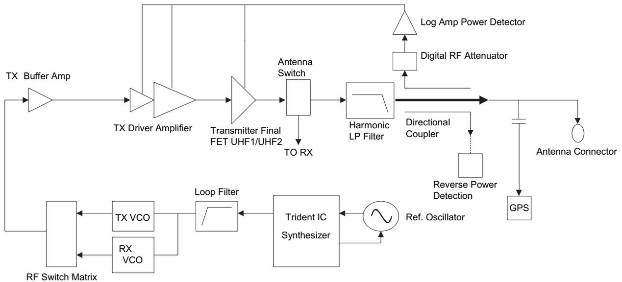
Figure 3-7. Transmitter (UHF1/UHF2) Block Diagram
