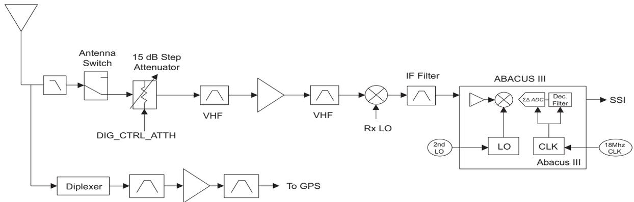
Figure 3-4. Receiver Block Diagram (VHF)
