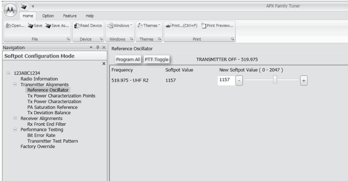
Figure 6-6. Reference Oscillator Alignment Screen (UHF2)
