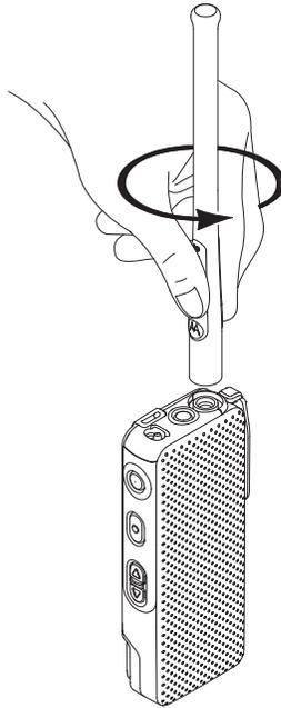
Figure 8-3. Removing the Antenna
