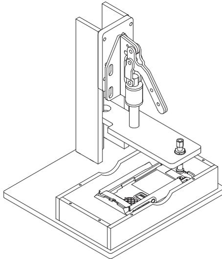
*Figure 8-30. Attaching Vacuum Test Fixture*
