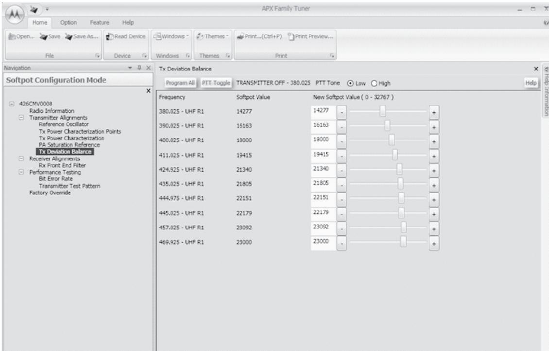
Figure 6-21. Transmit Deviation Balance Alignment Screen (UHF1)
