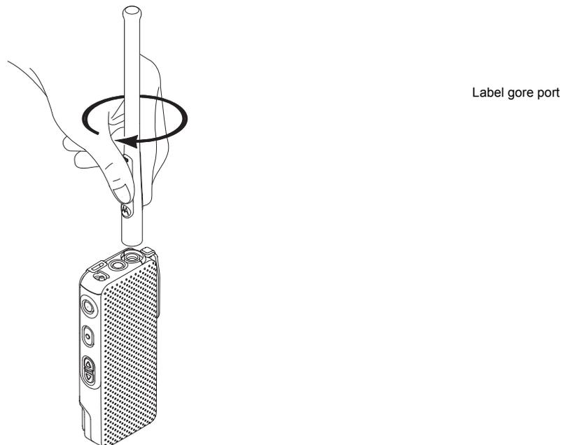
Figure 8-25. Attaching the Antenna
