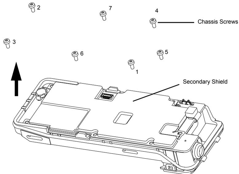
*Figure 8-8. Remove the chassis screws*
