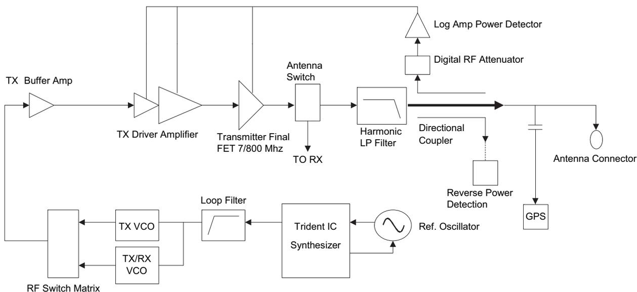
Figure 3-9. Transmitter (700/800 MHz) Block Diagram
