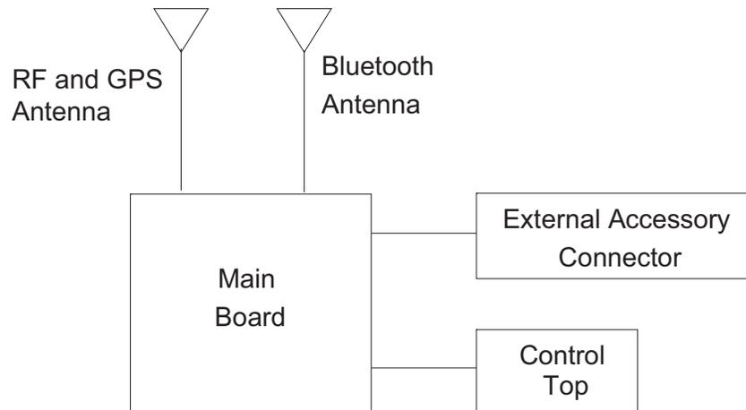
Figure 3-1. APX 3000 Overall Block Diagram
