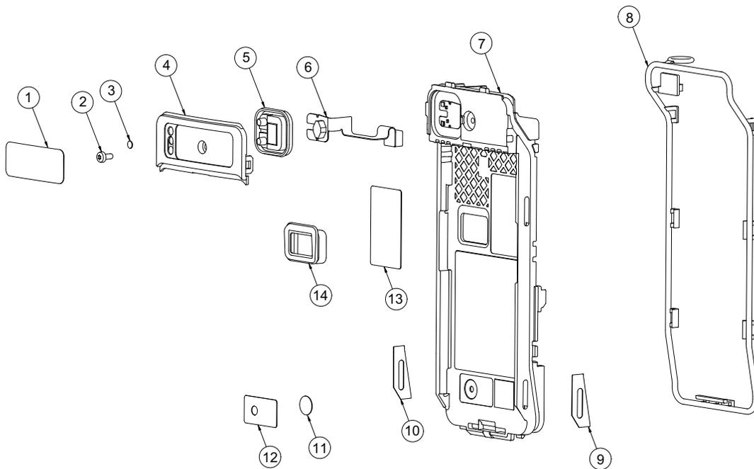
Figure 8-14. Serviceable Components – Chassis Assembly
