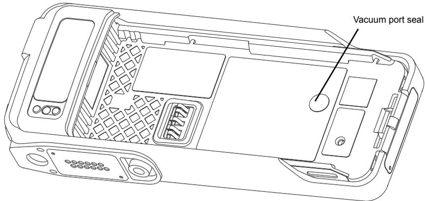
*Figure 8-26. Assemble the Seal, Vacuum Port*
