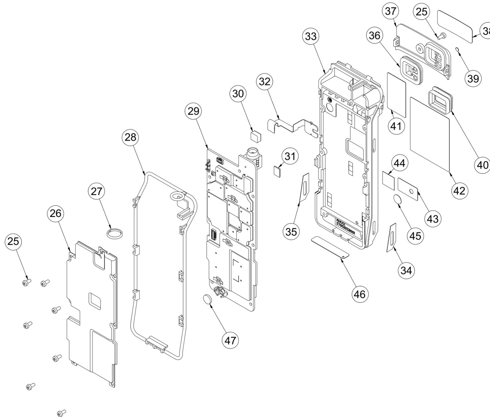
Figure 10-2. APX 3000 Back Kit Exploded View
