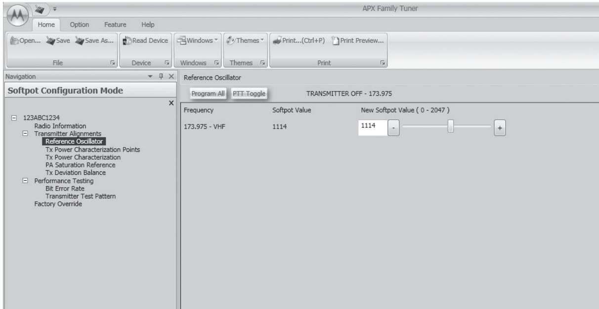
Figure 6-7. Reference Oscillator Alignment Screen (VHF)
